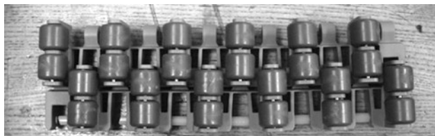
Figure 189: Assemble in two-row increments
