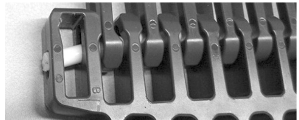
Figure 331: Insert rod through hinges
