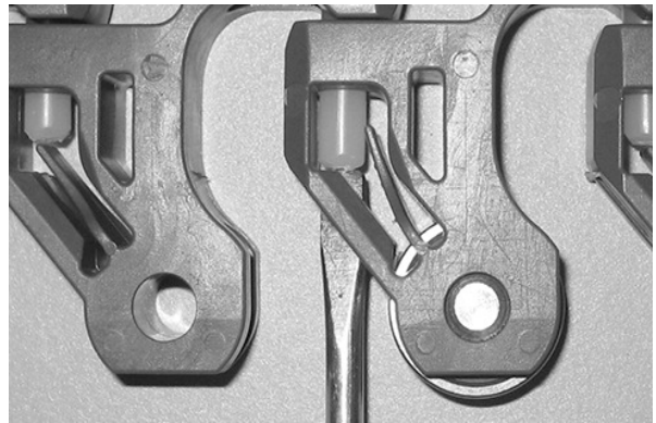
Figure 300: Push rod past retention feature
