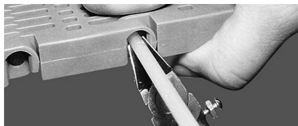
Figure 39: Cut rod flush with belt edge
