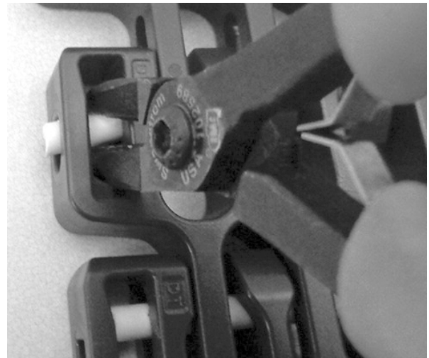
Figure 316: Push rod to side and past hole
