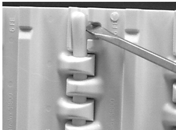
Figure 206: Lift rod over retention feature
