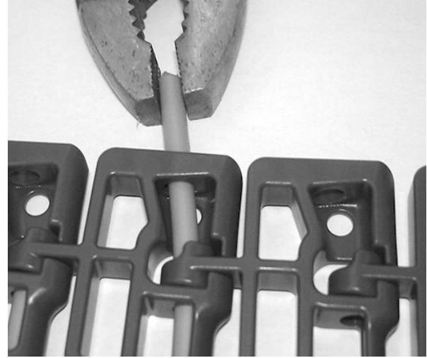
Figure 126: Pull rod from belt
