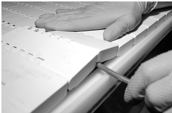
Figure 88: Slightly bend and insert rod through hinges
