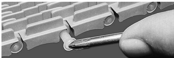
Figure 22: Push rod into belt
