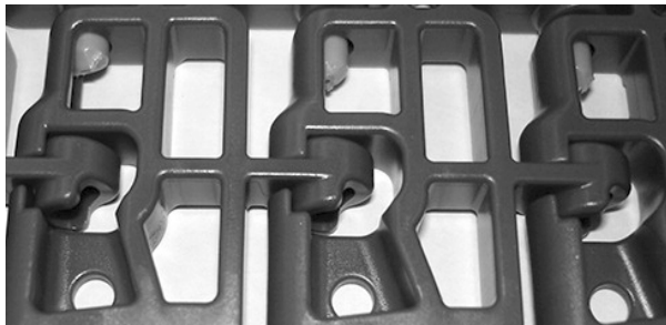
Figure 116: Rods move inside flush edge
