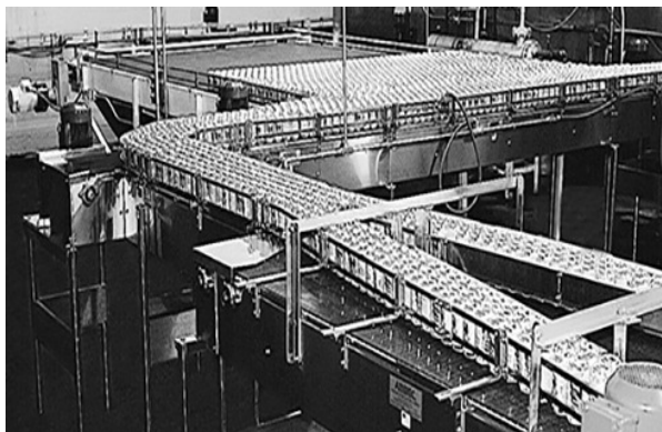
Figure 17: Place supports across width of belt
