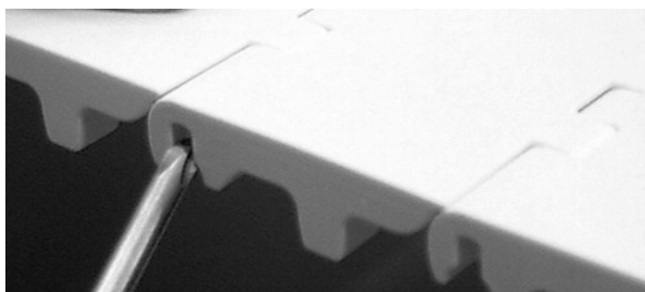
Figure 204: Push rod past retention figure
