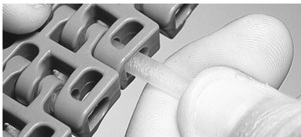
Figure 144: Insert rod through hinges
