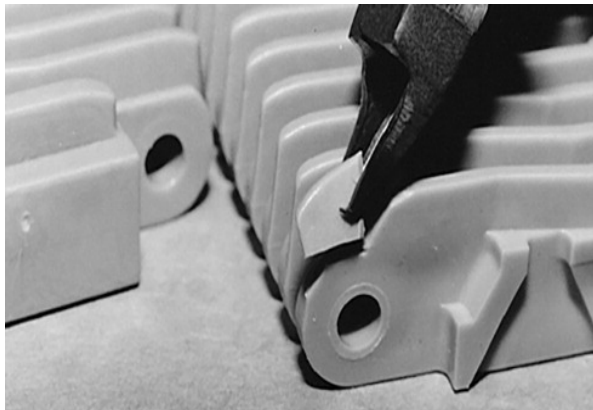
Figure 47: Cut outermost rib
