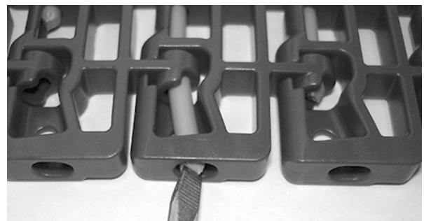
Figure 123: Push rod past retention feature
