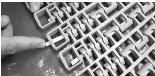
Figure 338: Push rod past retention feature
