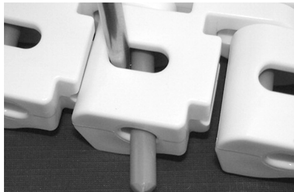
Figure 285: Push rod through retention feature
