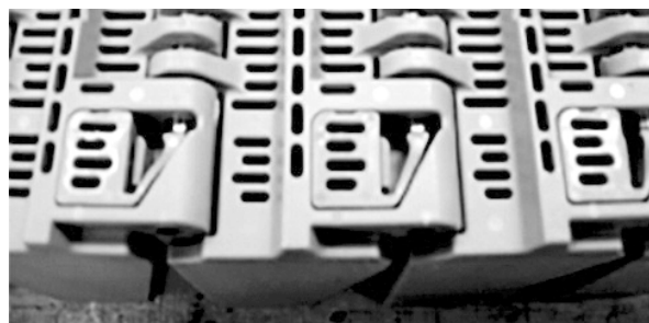
Figure 105: Ensure retention feature is closed
