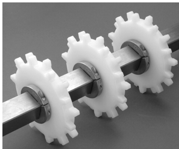
Figure 318: Secure both sides of all sprockets
