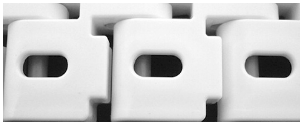
Figure 284: Ensure rod is past retention feature
