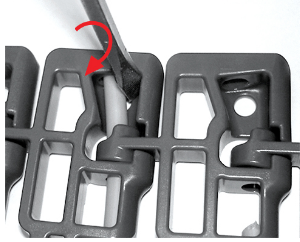
A Retention feature Figure 125: Push rod past retention feature
