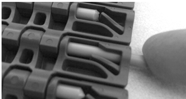
Figure 127: Insert rod through hinge
