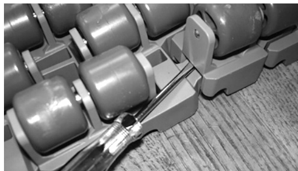
Figure 192: Insert screwdriver under roller
