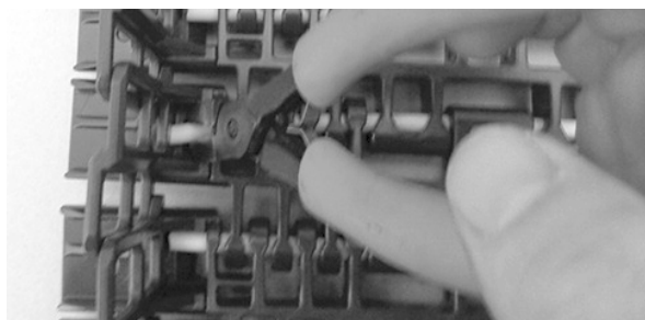
Figure 367: Push rod past retention feature
