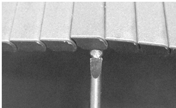
Figure 54: Push rod head past retention feature
