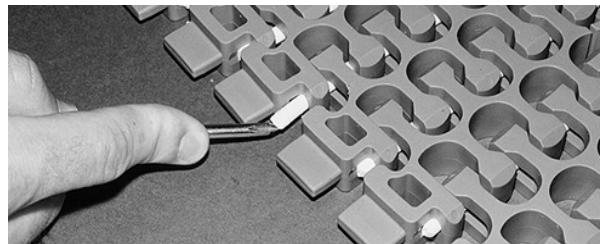
Figure 271: Ensure rod is past retention feature
