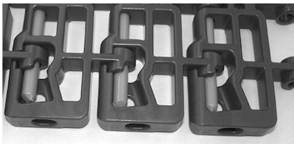
Figure 117: Rod grows into flush edge
