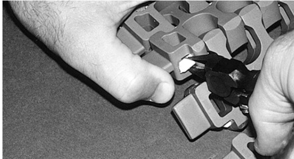
Figure 273: Free rod from retention feature
