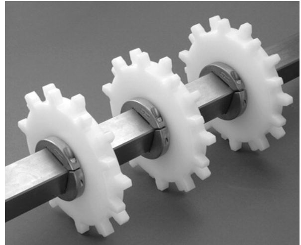
Figure 335: Secure both sides of all sprockets
