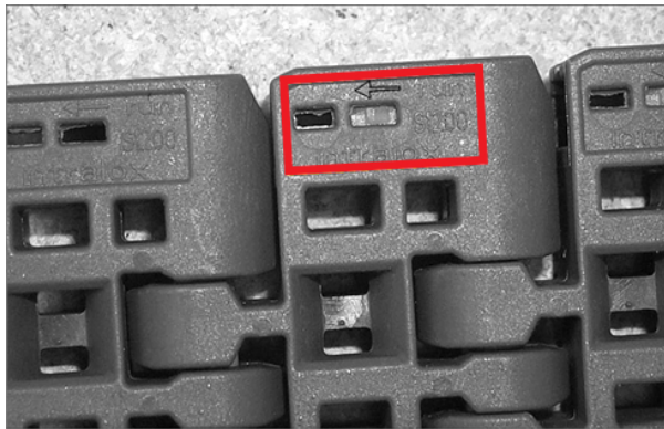
Figure 154: Belt running direction
