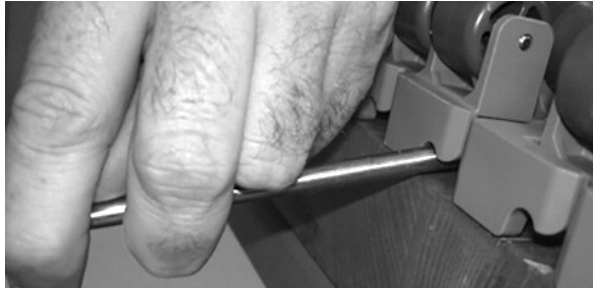
Figure 193: Insert steel pin in hinge
