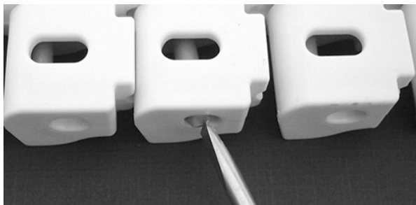
Figure 283: Push rod past retention feature
