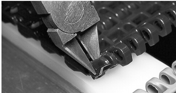
Figure 140: Cut off half of edge
