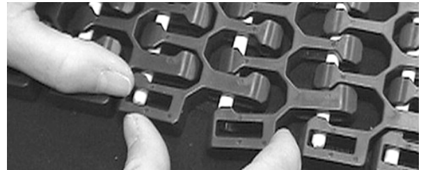
Figure 307: Push rod past belt edge, snap flush edge over rod
