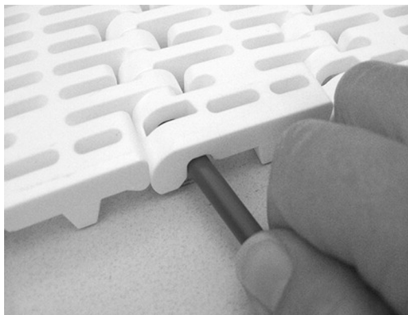
Figure 79: Push rod into belt
