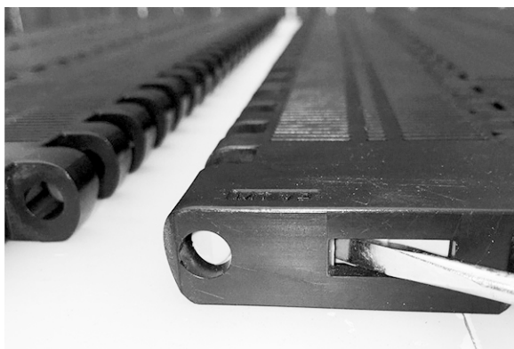
Figure 209: Use screwdriver to close Slidelox
