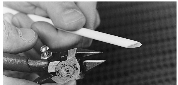
Figure 14: Clip rod at angle
