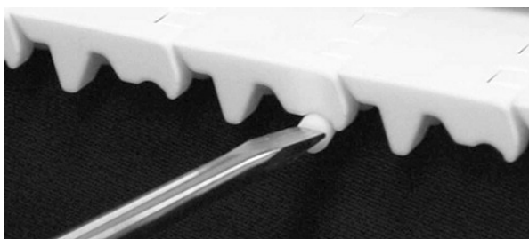
Figure 174: Push rod past retention feature
