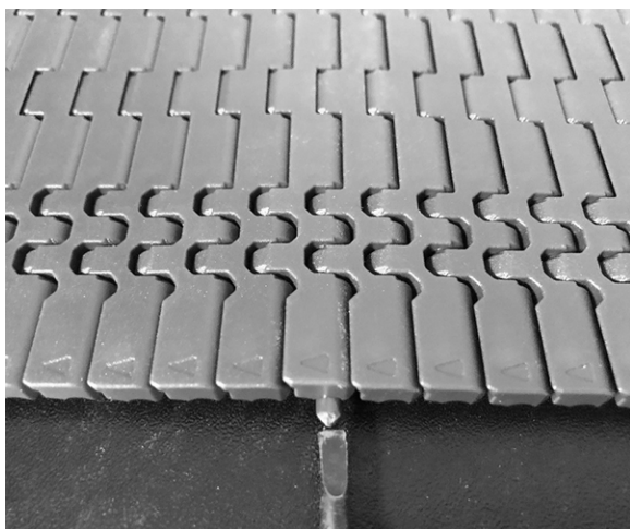
Figure 59: Push rod past retention feature
