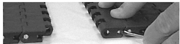
Figure 160: Use screwdriver to close Slidelox
