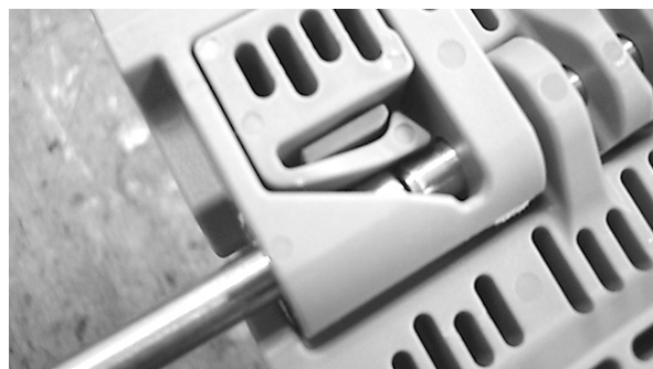
Figure 104: Push rod past retention feature
