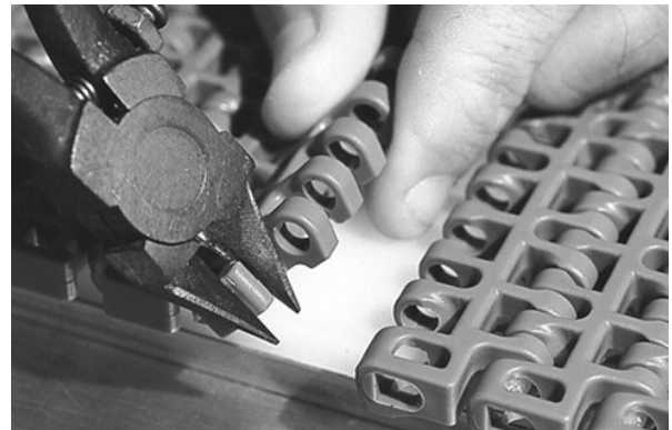
Figure 142: Cut edge from belt
