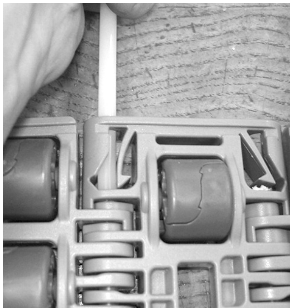
Figure 221: Push rod from belt
