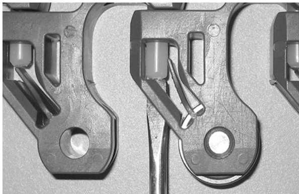
Figure 278: Push rod past retention feature
