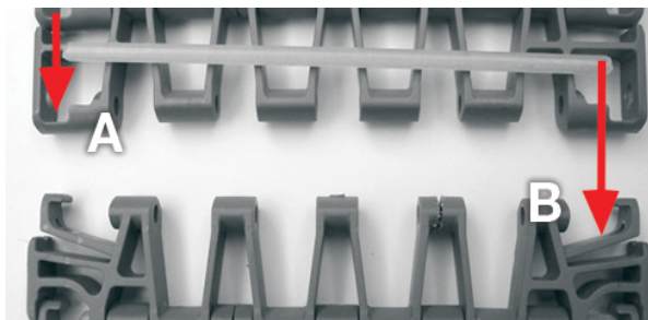
A Original belt section B New belt section
