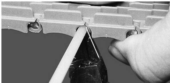
Figure 24: Cut rod flush with belt edge
