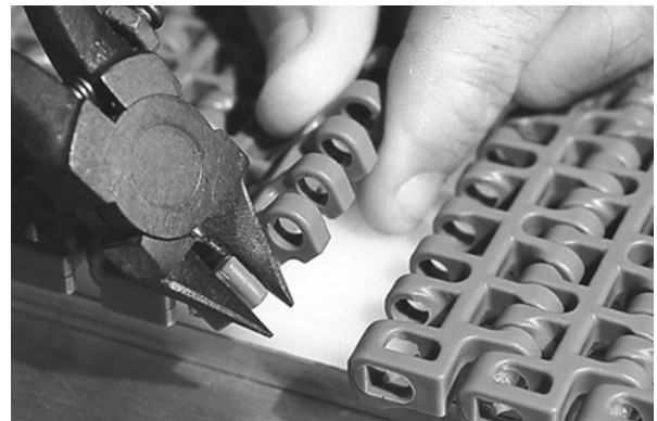
Figure 152: Cut edge from belt
